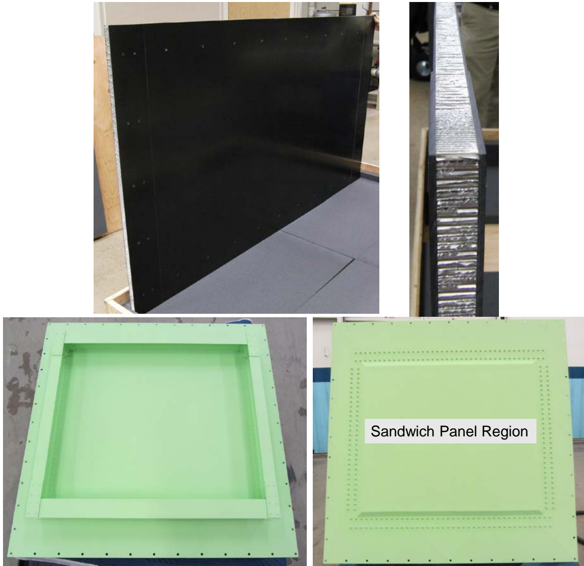
Figure 1. Launch vehicle panel (top) with free boundary conditions, and rotorcraft roof panel (bottom) simply supported between a frame structure.
