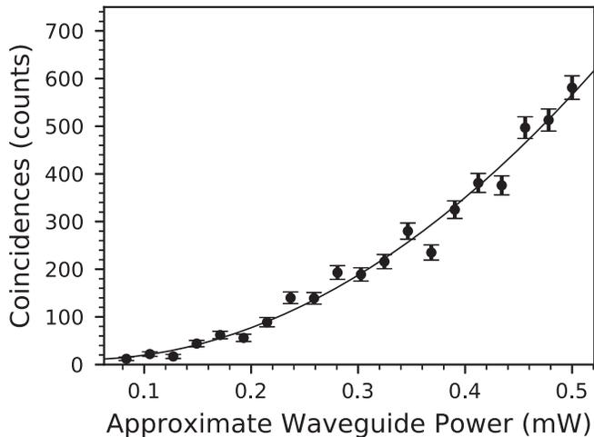
FIG. 3. The input pump power is varied and coincidences are measured, exhibiting the quadratic behavior of the device. Error bars enclose one standard deviation. Input waveguide power is approximated based upon loss measurements. Values above 0.5 mW begin to saturate the quadratic pair generation rate.
