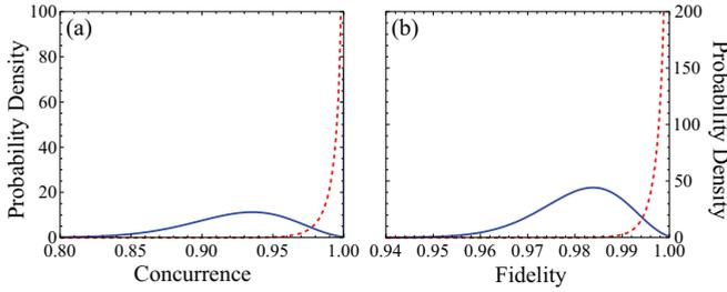
FIG. 2. (Color online) Probability distribution of the (a) concurrence and (b) fidelity of an ensemble of qubits subjected to a random disturbance before [solid (blue) line] and after [dashed (red) line] measurement reversal. The disturbance is quantified by a Gaussian random variable with mean  $\phi_a = \pi/8$  and standard deviation  $\sigma = \pi/30$ .
