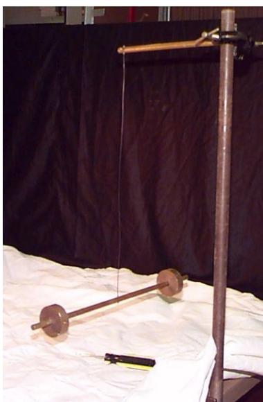
The rod is suspended from a thin wire. As the rod rotates in the horizontal plane, the wire twists and gently pulls the rod back. While springs are good at measuring medium and big forces, torsion balances let you measure tiny forces, most notably used in 1798 to measure the mass of the Earth.
