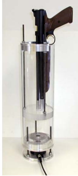
Figure 1. Air-gun based blunt impact system
