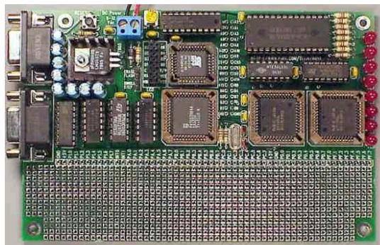
The two 8052 internal serial ports are designed and configured as RS232 serial communications ports that provide for connections to a PC using a terminal emulation such as window's "Hyper-terminal". In this way, programs are written using a text editor, then assembled, and downloaded into RAM or FLASH ROM using the MONITOR utility. For more information on the board and software details, visit the PJRC homepage<sup>2</sup>.
