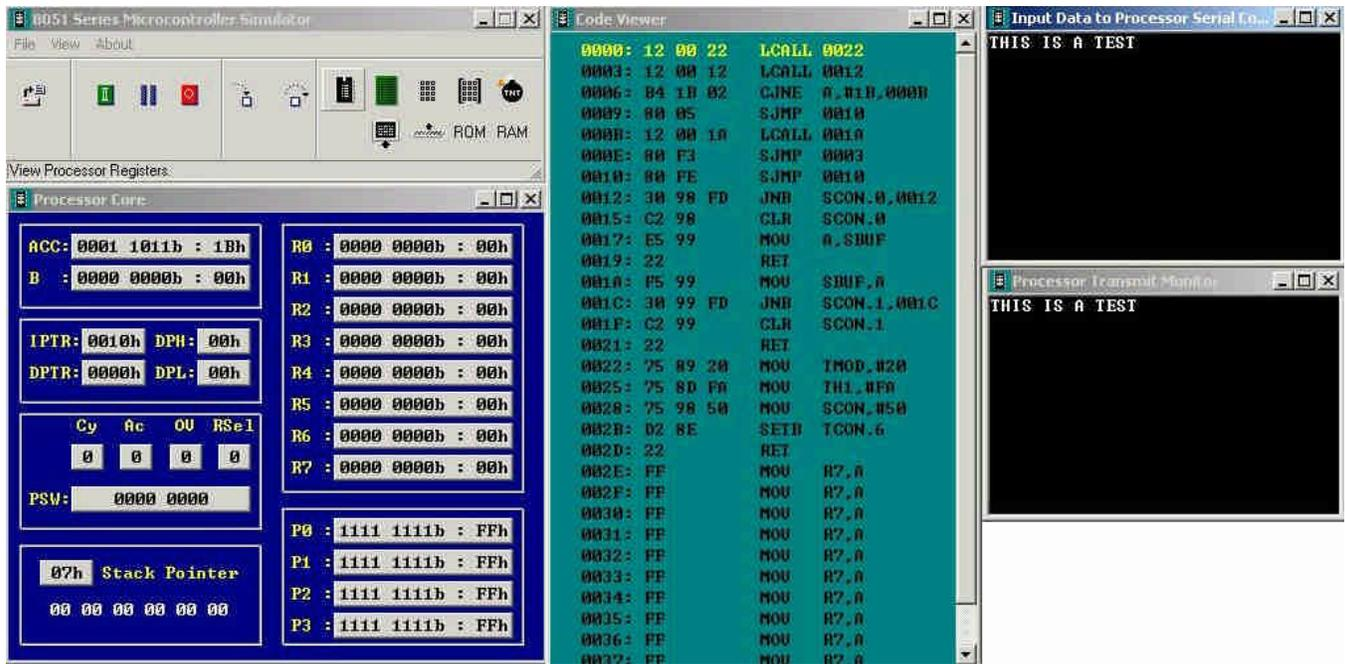
Notice that the simulator interface shows all the 8051 registers, flags, ports and provides simulated keyboard and terminal interfaces via the SBUF register. For example the image above shows the simulator loaded and running a program the reads the simulator keyboard buffer and sends the ASCII value to the simulator display until the “ESC” key is pressed. With minor modifications this program can be loaded onto the Micro-controller board and run in lab.
