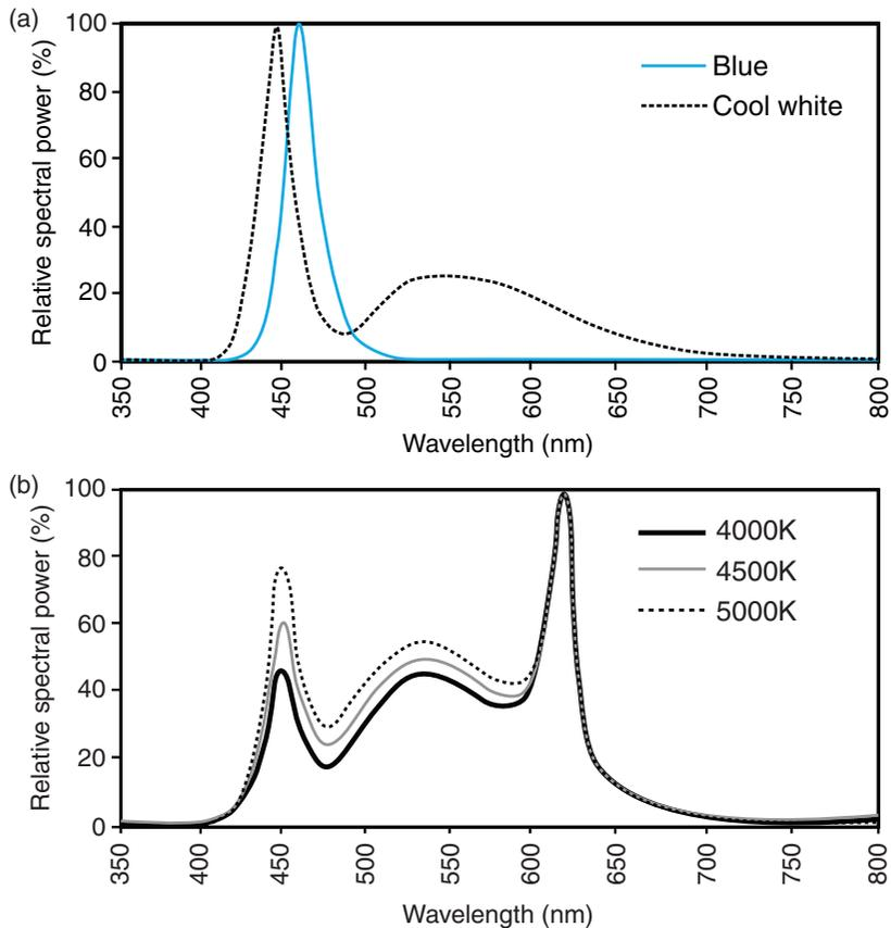
**Figure 2** Relative spectral power distributions of the cool-white light and blue light desktop luminaires (top) and overhead lights (bottom) used in this study. The overhead luminaires were used at the FHWA site only
