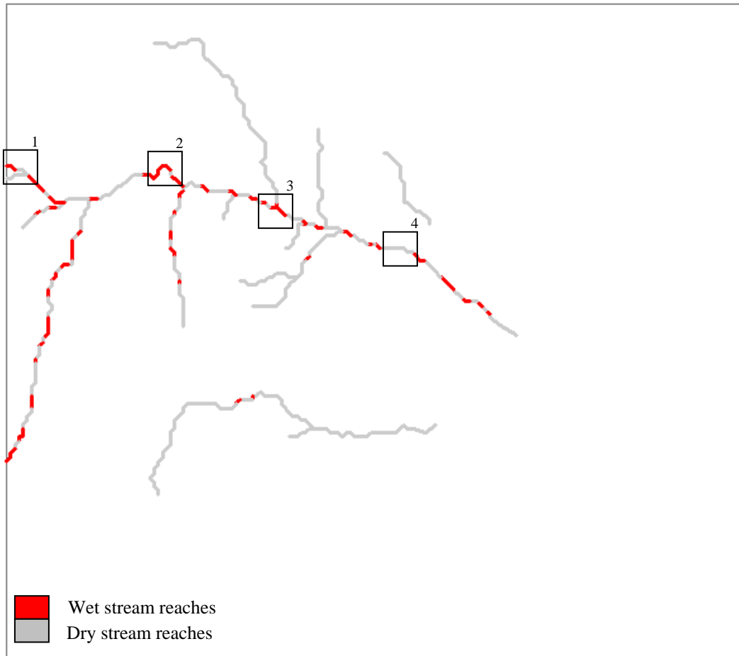
Fig. 12: Wet-dry areas obtained from steady-state simulation of Rio-Salado basin using ModHMS (Beeson, 2008)
