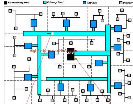
A typical VAV supply ductwork layout (air terminals)<sup>2</sup>
