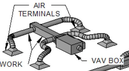
A typical layout of a VAV box and diffusers (air terminals)<sup>3</sup>
