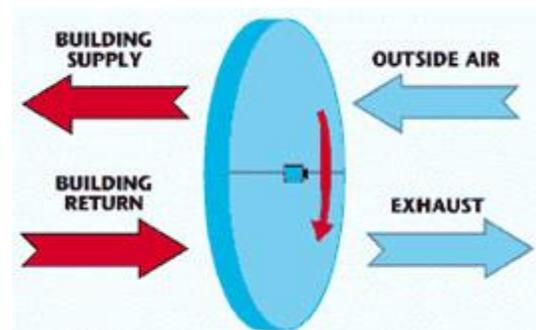
A diagram of a typical energy recovery wheel<sup>4</sup>
