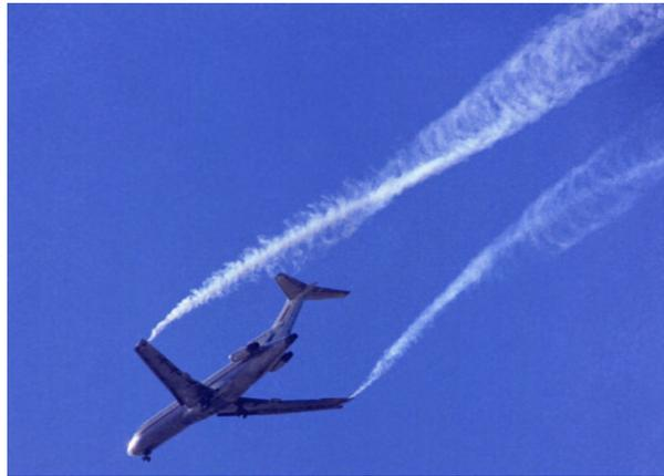
**Fig. 4.** B-727 vortex study photo (Courtesy: NASA Dryden Flight Research Center)
