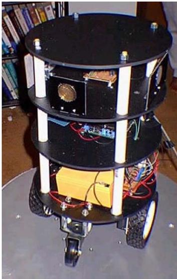
Figure 3. Zagros Max99 mobile robot with 12 inch diameter platforms [from Ref. 3]
