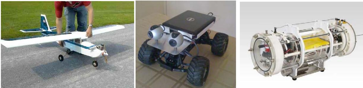
Figure 1. Examples of Penn State's unmanned air-, ground-, and underwater vehicles.
