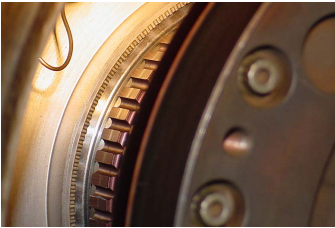
Figure 2A. 60 tooth gear encoder installed on high speed turbo machinery.
