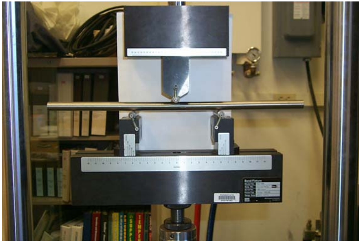
Figure 2. Shaft specimen in three point bending MTS fatigue machine.
