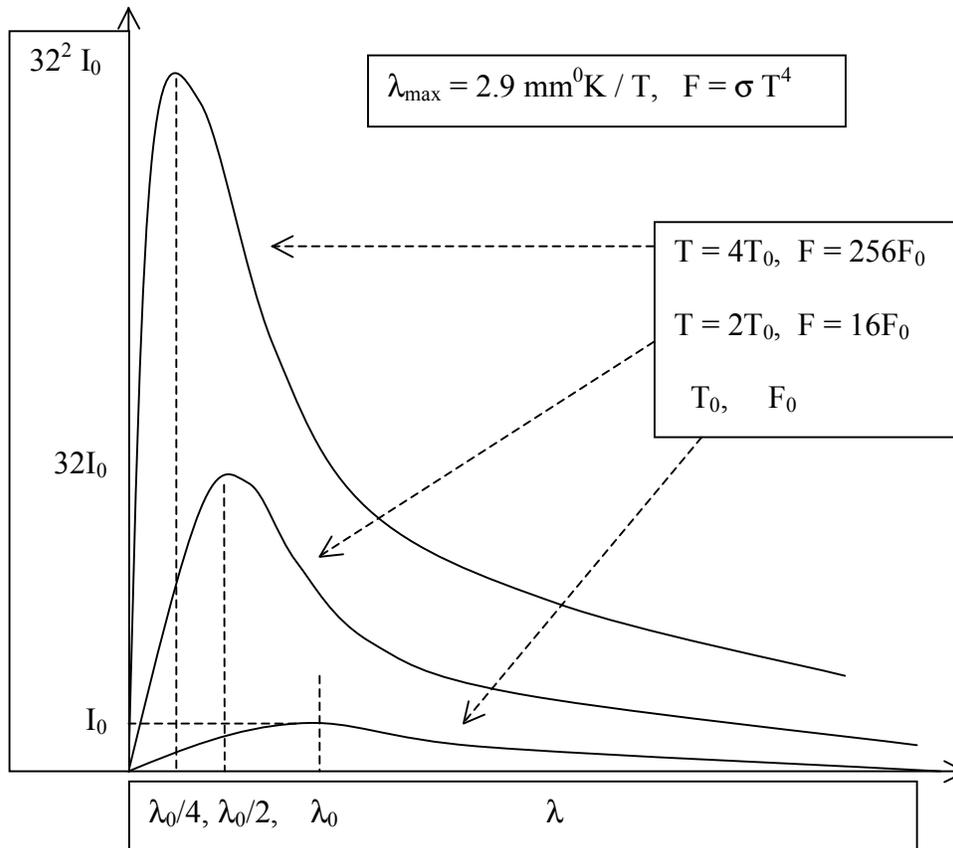
**Fig. III.1:** Thermal (Black Body) radiation curves for surfaces of various temperatures.
