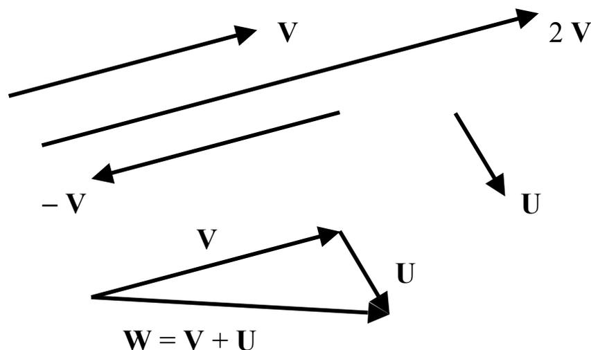
**Fig. 1:** Representing directed magnitudes (vectors) by arrows and the algebraic manipulation of arrows.
