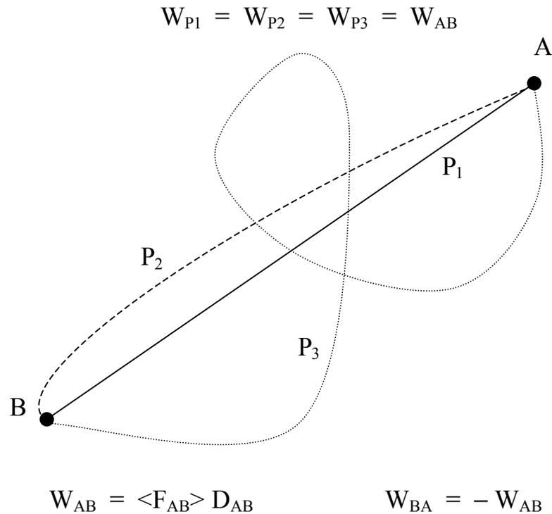
**Fig. 4:** The work done by a conservative force acting on an object moving from one point, A, to another point, B, does not depend on the path taken by the object, but just on the endpoints, A and B.
