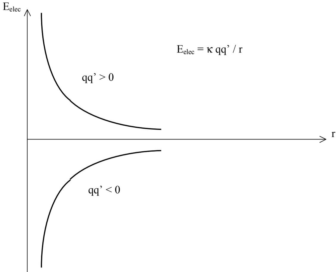
**Fig. 9:** Electrostatic potential energy curves for  $qq'$  positive or negative.
