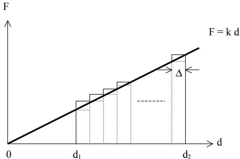
**Fig. A3:** Graph of the force,  $F$ , (vertical axis) required to stretch a spring against the length of the stretch,  $d$ , (horizontal axis). The vertical rectangles are referred to in the discussion below.
