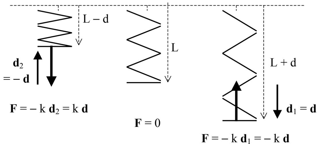
**Fig. 7:** Forces exerted *by* a stressed spring
