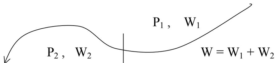
**Fig. 3b:** Path,  $P$ , regarded as composed of two parts,  $P_1$  and  $P_2$ , in which the varying force does work  $W_1$  and  $W_2$ , respectively.
