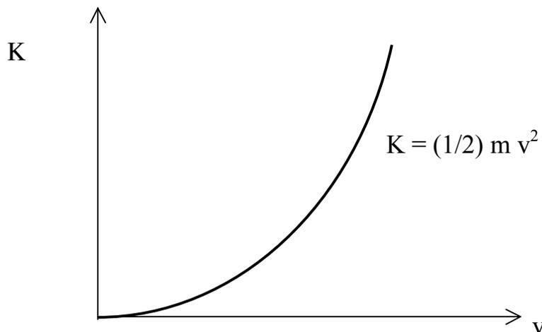
**Fig. 11:** The dependence of kinetic energy on speed
