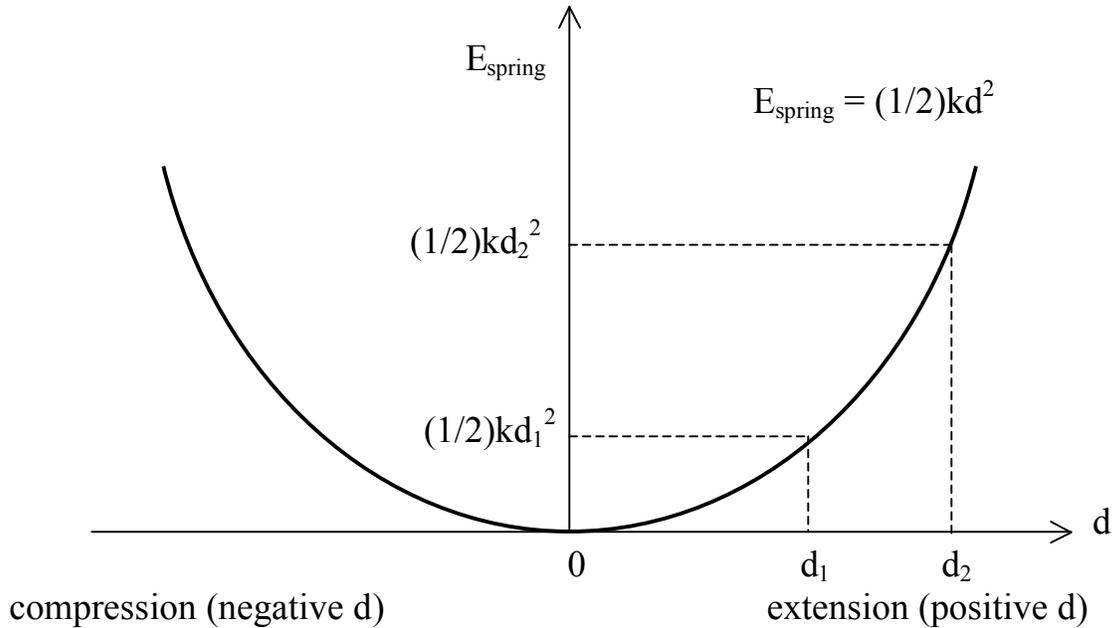
**Fig. 8:** Elastic potential energy curve, relative to the relaxed state, for a spring of stiffness,  $k$ .
