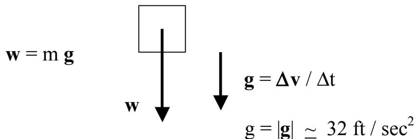
**Fig. 10:** The relationship between weight and mass near Earth's surface. If the weight,  $w$ , is the resultant force, then the object falls with the universal acceleration,  $g \simeq 32 \text{ ft} / \text{sec}^2$ .
