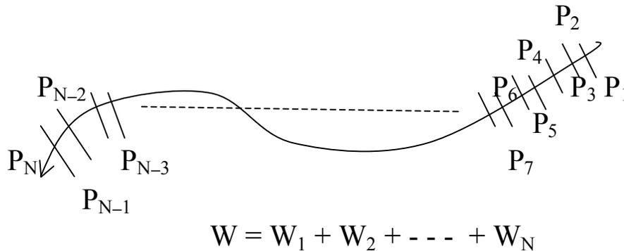
**Fig. 3c:** Path,  $P$ , broken up into a large number,  $N$ , of almost straight, short paths in each of which the force is almost constant. Work,  $W_n$  is done in the part,  $P_n$ .
