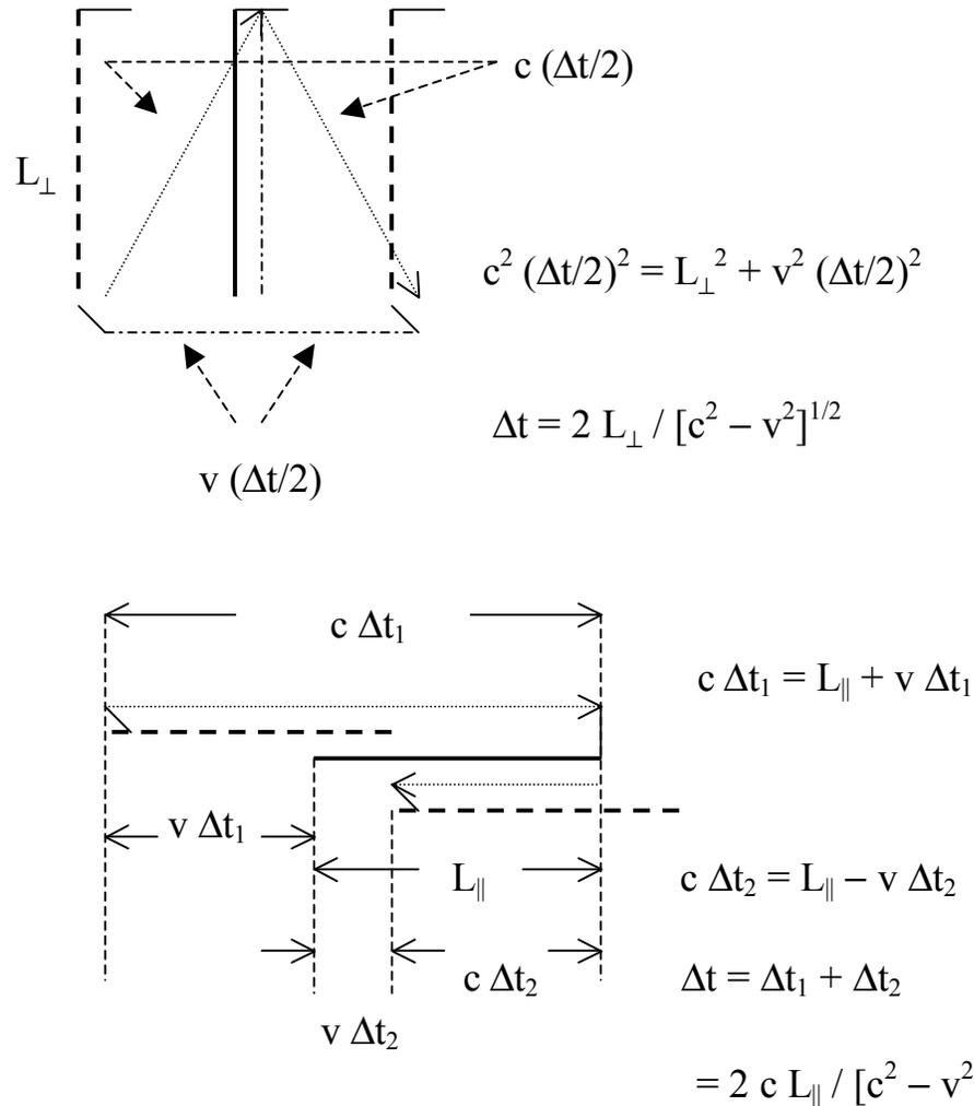
**Fig. 1.2:** The light clock from the perspective of the inertial frame,  $F$ , in which the clock moves with speed,  $v$ , to the left. The top diagram describes the motion of the vertical rod and the up and down light pulse path. The bottom diagram describes the motion of the horizontal rod and the right and left light pulse path.
