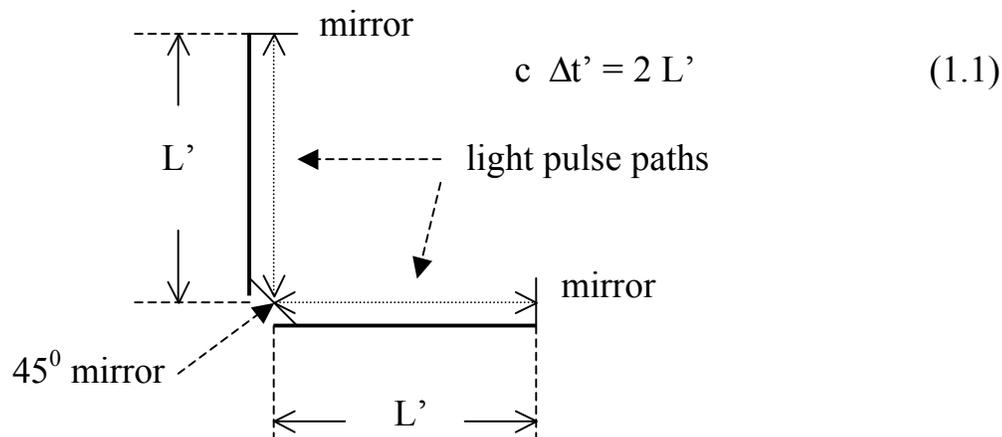
**Fig. 1.1:** Structure of light clock from the perspective of its rest frame,  $F'$ . The time interval between consecutive reflections from the  $45^\circ$  mirror at the join of the vertical and horizontal rods is  $\Delta t'$ .
