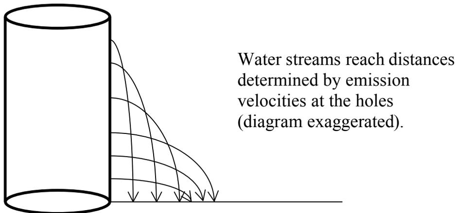
**Fig. IV. 3:** Water streams from small holes in full container at different depths below water surface.
