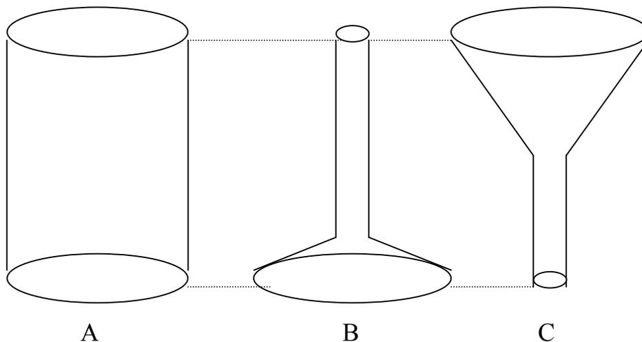
**Fig. IV. 5:** Hydrostatic pressure 'paradoxes'.
