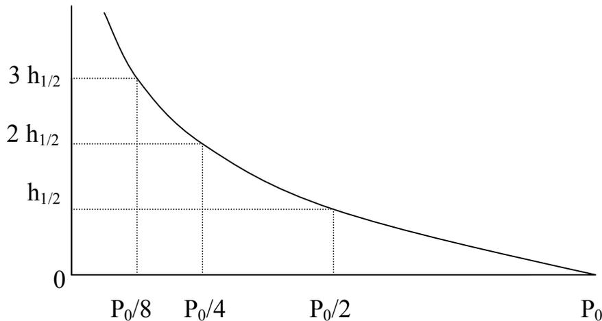
**Fig. IV. 7:** Exponential drop in air pressure with height
