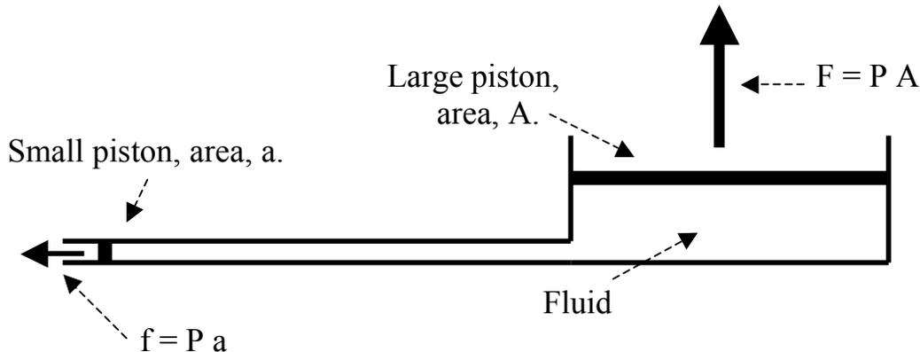
**Fig. IV. 6:** The hydraulic lift
