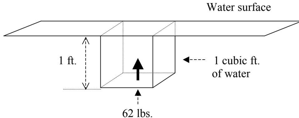
**Fig. IV. 1:** Water pressure supporting (balancing) water weight
