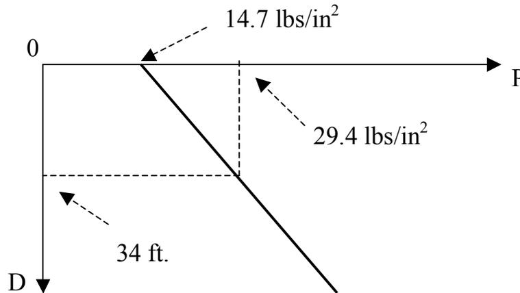
**Fig. IV. 2:** Graph of linear (straight line) variation of pressure with depth in water according to the equation,  $P = [(0.43 \text{ lbs/in}^2)/\text{ft}] D + 14.7 \text{ lbs/in}^2$ .
