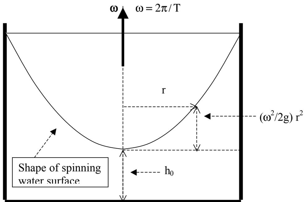
**Fig. IV. A2:** Parabolic surface of water spinning with paint can container
