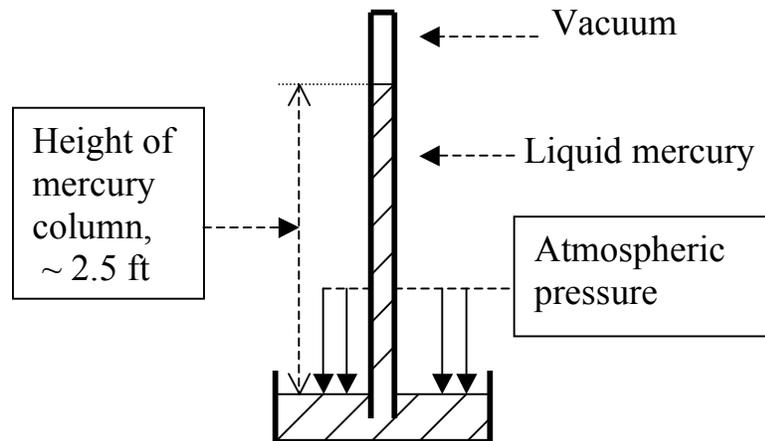
**Fig. IV. 13:** The basic barometer
