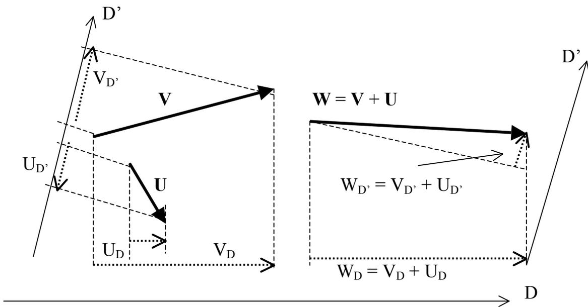
**Fig. I. A3:** Algebraic relations between vectors and their components in two directions. In this example all the algebraic components along directions  $D$  and  $D'$  are positive except  $U_{D'}$ , which is negative.
