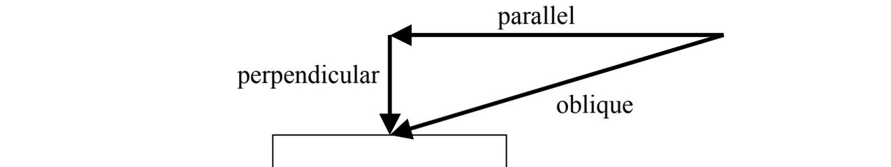
**Fig. I. 5a:** Components of oblique force applied to object on floor.
