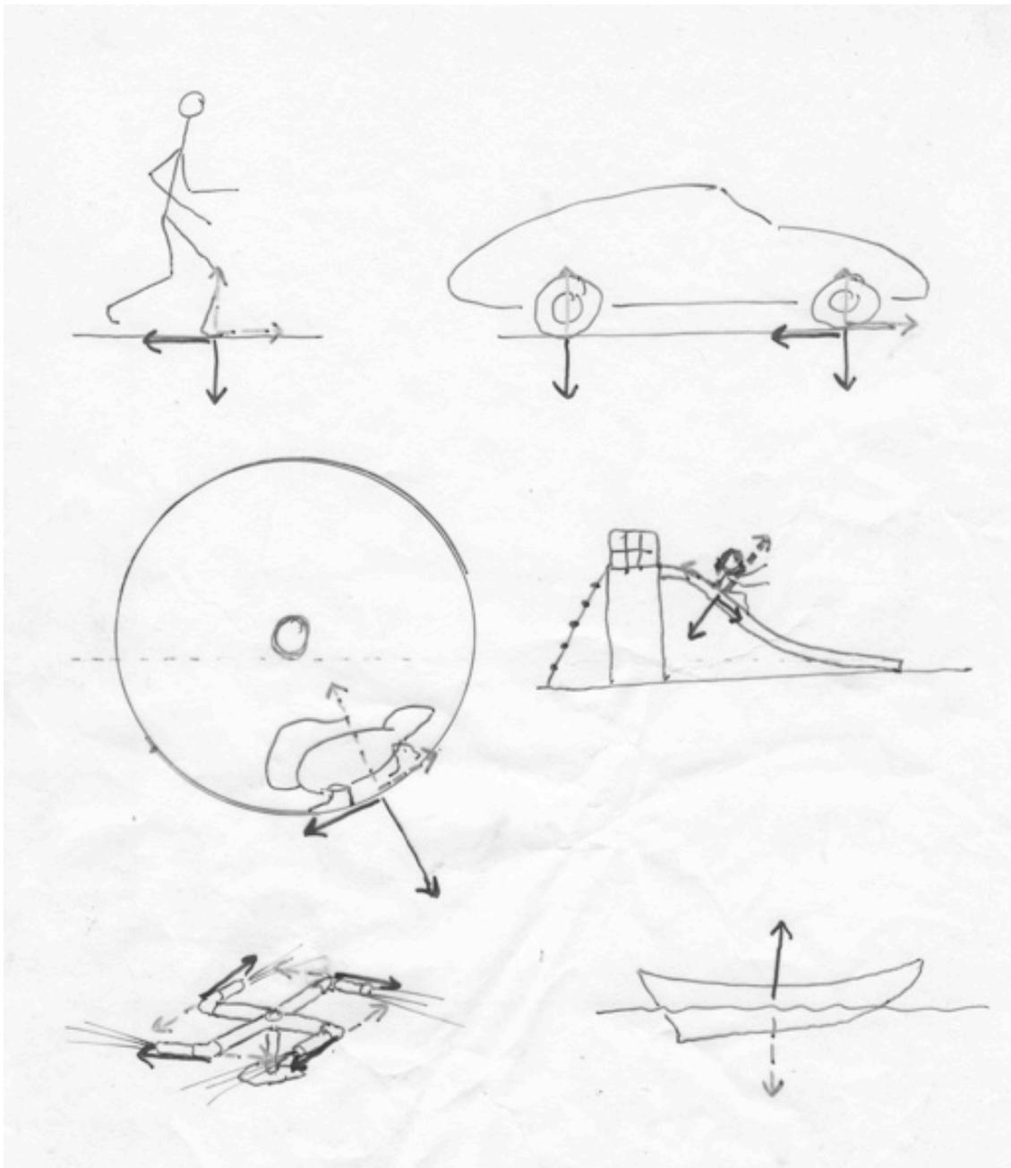
**Fig. I. 1:** Action – reaction force pairs. Action (bold) – reaction (light).
