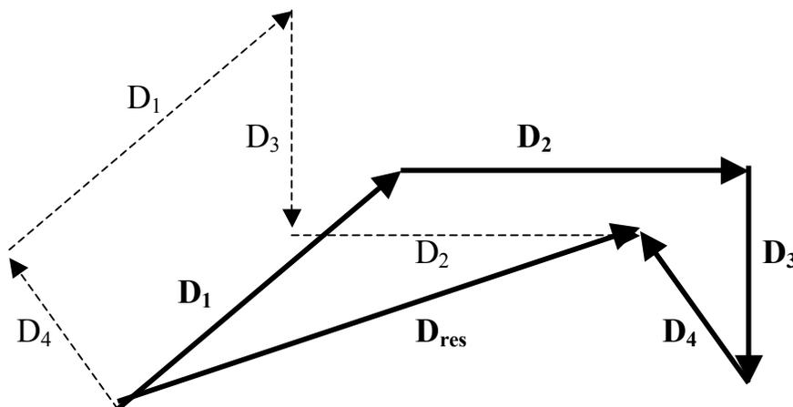
**Fig. I. 4:** Resultant of several displacements (or several forces). Note the independence of the resultant on the order of composition.
