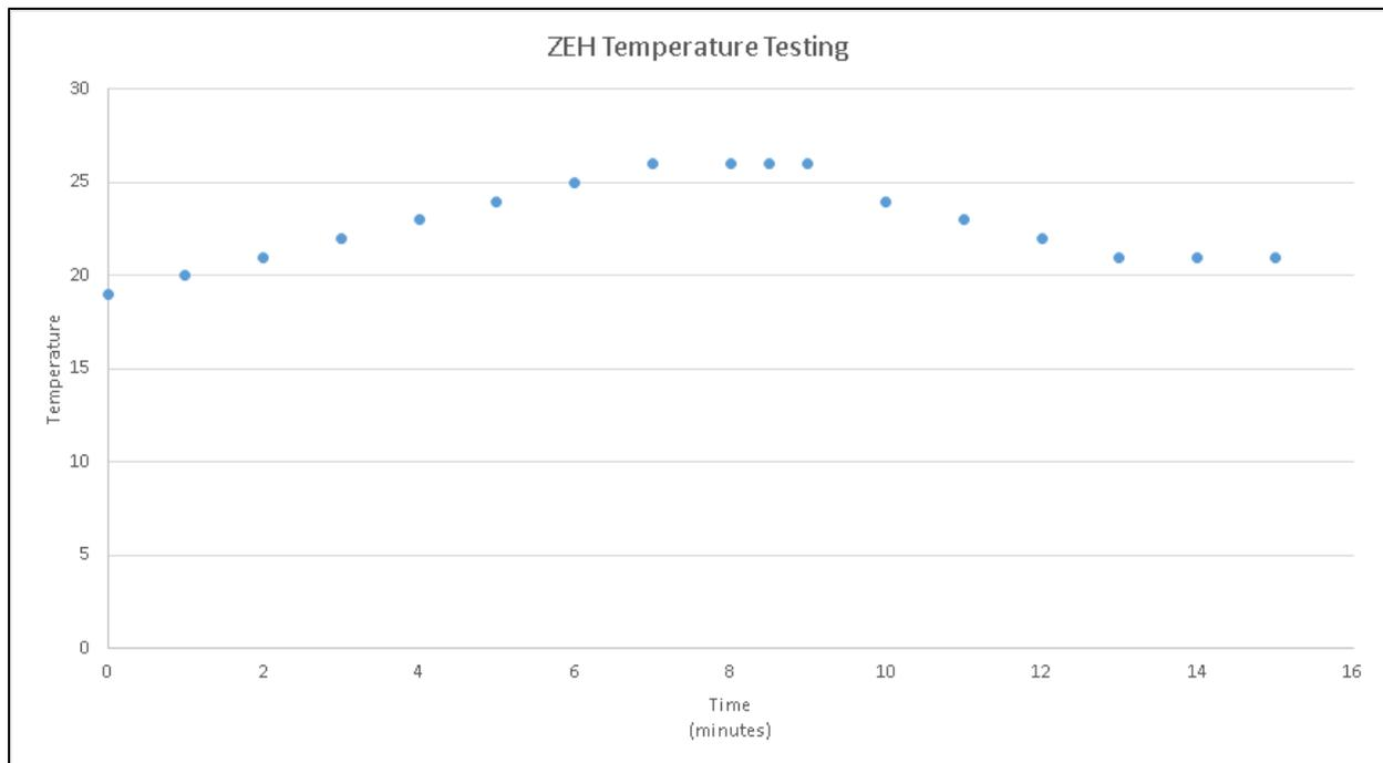
The temperature of the house was tested with a probe. The south side of the house was exposed to a light bulb for eight minutes simulating how the sun would be absorbed to warm the house. The house was then removed and exposed to a fan with a bucket of ice in front of it for the remaining time. The fan simulated the wind throughout the night. The temperature was monitored and then recorded.
