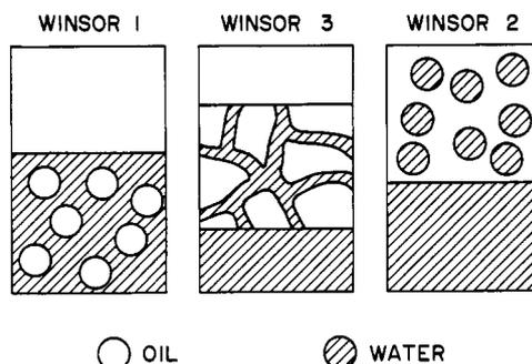
Figure 1. Schematic representation of Winsor 1, Winsor 2, and Winsor 3 microemulsion systems. Winsor 1 and Winsor 2 systems are characterized by spherical droplet microstructures and two coexisting phases. Winsor 3 system is characterized by bicontinuous microstructure and three coexisting phases.
