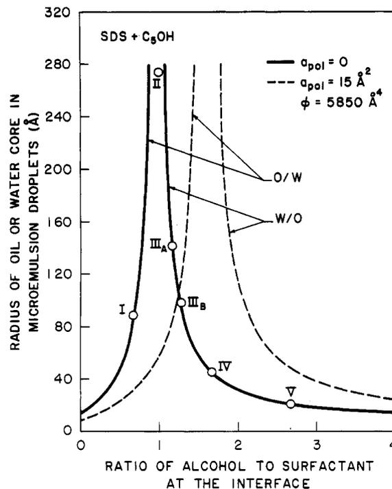
**Figure 4.** Radii of the film-water and film-oil interfaces in microemulsion droplets. Continuous line refers to the polymer-free droplets while the dotted line refers to the polymer-bound droplets. The system is identical to that in Figure 3 and the five points marked here correspond to those in Figure 3.
