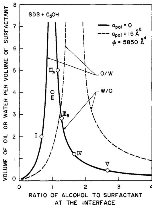
**Figure 3.** Volume ratio of the dispersed phase (oil or water) in the microemulsion droplet to the surfactant in the film region of the droplet. Continuous lines refer to the polymer-free droplets while the dotted lines refer to the polymer-bound droplets. See text for a discussion of the five points indicated in the figure which correspond to the five types of allowed structural transitions.
