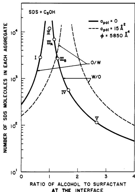
**Figure 5.** Number of surfactant molecules contained within the film region of the microemulsion droplet. Continuous lines refer to the polymer-free droplets while the dotted lines refer to the polymer-bound droplets. The system is identical to that in Figure 3 and the five points marked here correspond to those in Figure 3.
