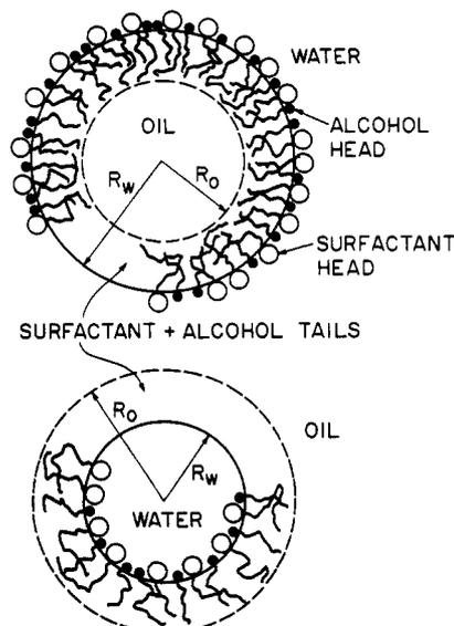
**Figure 2.** Microemulsion droplets of oil-in-water type and water-in-oil type indicating the different radii. The film region lies between the two radii.
