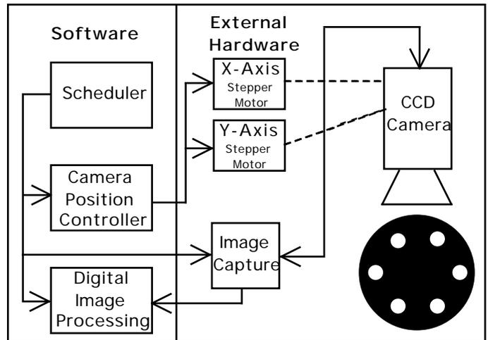
**Figure 1:** The behavior analysis apparatus is constructed from both software and hardware components; hardware is located outside the computer. The scheduling software module determines the timing of camera positioning, image capture, and processing of the digitized image. The camera is moved over each one of twelve dishes in the arena for image capture and processing.
