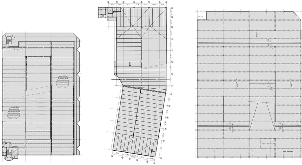
Figure 1. Plans at the same scale of the three case study parking garages (left to right): precast concrete, cellular steel and post-tensioned concrete.
