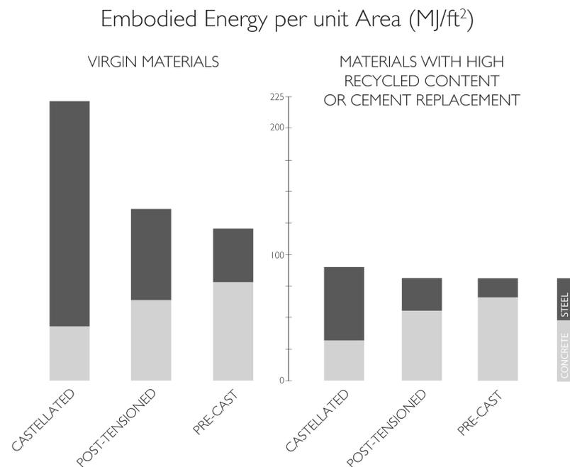
Figure 3. Cradle-to-gate embodied energy per square foot of floor area for each case study. Multiply by 10.8 to get MJ/m<sup>2</sup>.
