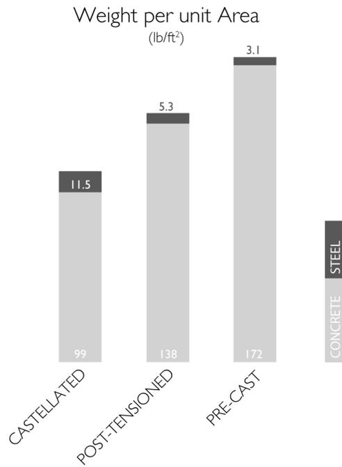
Figure 2. Structural material quantities per square foot of floor area. Multiply lb/ft<sup>2</sup> by 4.88 to get kg/m<sup>2</sup>.
