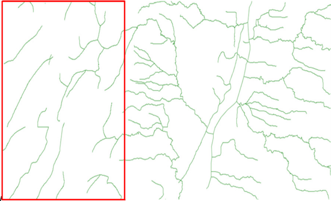
Figure 7: Comparison of generalized NHD to non-generalized NHD. This could be viewed as the scale change from 1:200,000 (left) to 1:50,000 (right)
