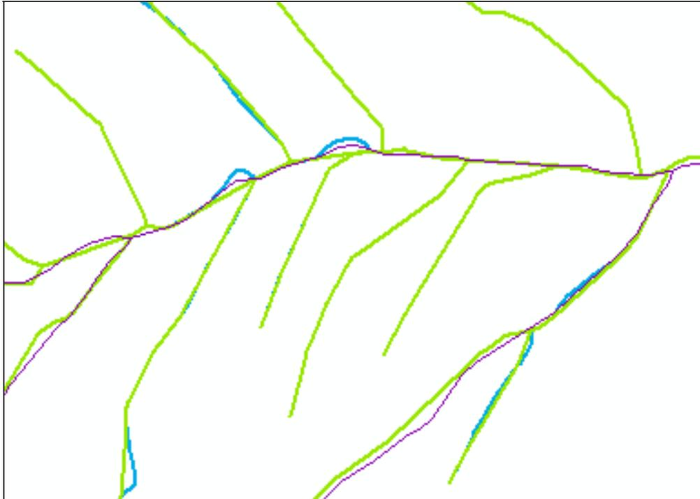
**Figure 7.** Colorado flowline data generalized for use at 1:100,000 scale with the ladder approach (blue) and the star approach (green), along with the original NHD medium resolution data (purple). Shown at an exaggerated 1:24,000 scale.
