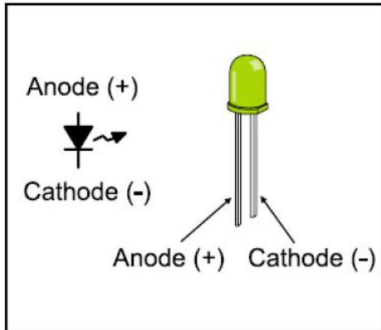
How do we know which lead is the Anode and which is the Cathode? There are two ways:
