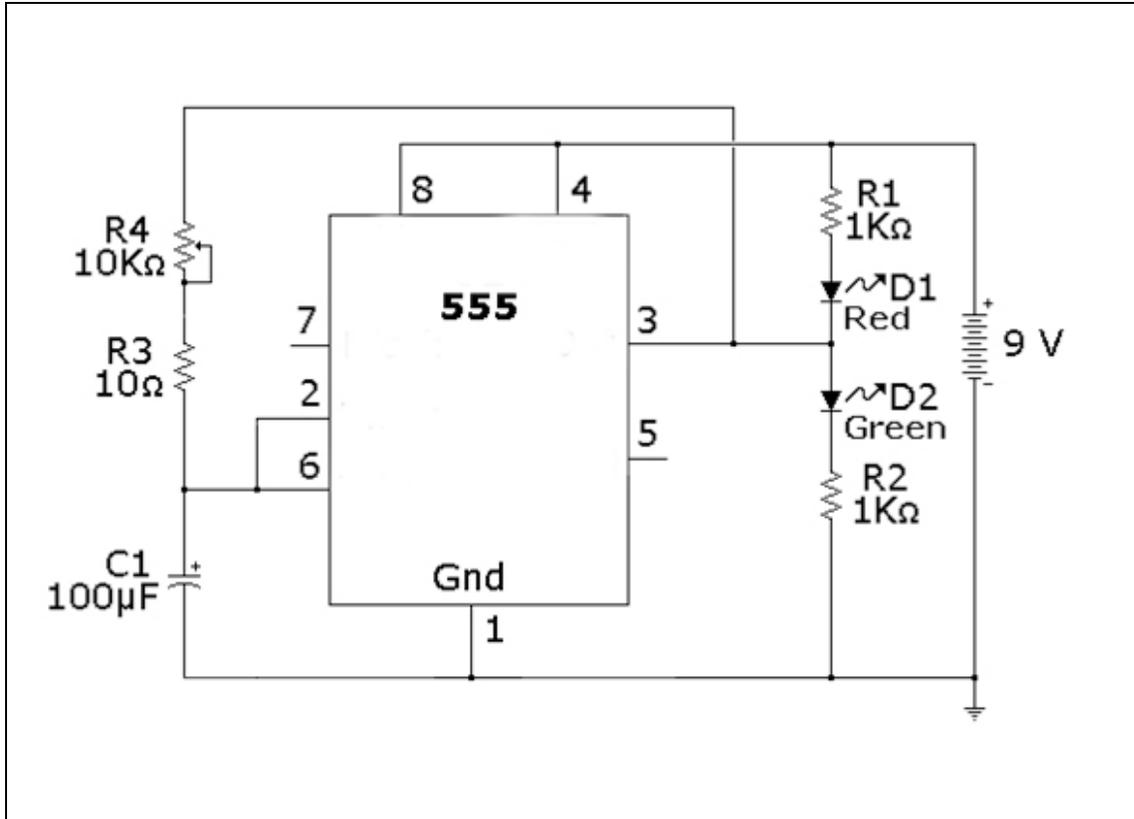
To verify that the circuit is working correctly, changing the value of the potentiometer R4 should result in a change in the frequency at which the LEDs are blinking. If you want you can connect a piezoelectric speaker to pin 3 to have an auditory output.
