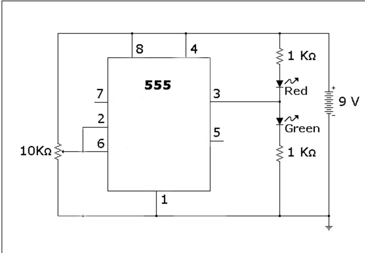
Connect the DMM to Pin 6 of the 555 IC. This is the Trigger Pin and indicates the voltage that makes the IC to change states.
